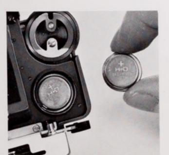
To replace weak or worn-out batteries, unscrew the cap over the battery chamber using a coin or key and the batteries will drop out. Make sure that the positive (+) side faces out when new batteries are installed.
