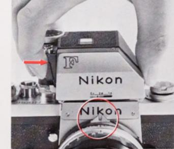
To remove the finder, depress the finder lock lever and press the finder release button located on the back of the camera. The finder will be unlocked and can be lifted out.
