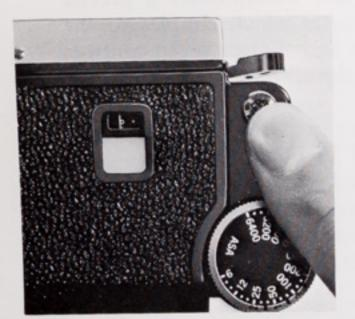
The Photomic FTN Finder is powered by two 1.3 volt mercury batteries located in the battery chamber on the bottom of the finder. To check the batteries, press the meter switch-off button and observe the needle in the window on top of the finder. If the needle swings to the center circle or beyond, the batteries are in good condition. The two mercury batteries come installed with the Photomic FT<sub>N</sub> Finder.
